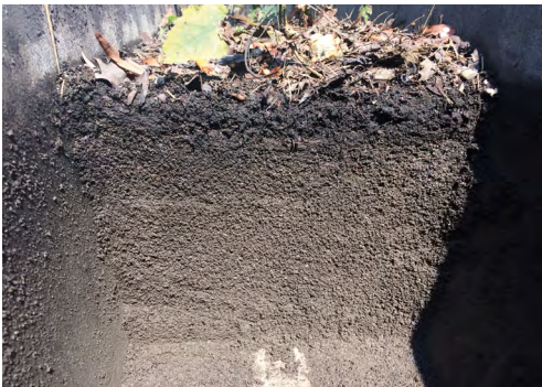
DRAINFIX CLEAN filter cake after 2 years of operation and a DTV of 24,000 vehicles - Munich, Germany
