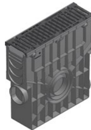
Trash box with plastic bucket, with ductile iron grating, black, SW 10 mm, class E 600, 4-fold bolted, 0,5 m
