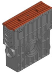
Trash box with PE mud bucket and FIBRETEC design slotted grating SW 9 mm, in the colour brick, class C 250, locked, 0,5 m
